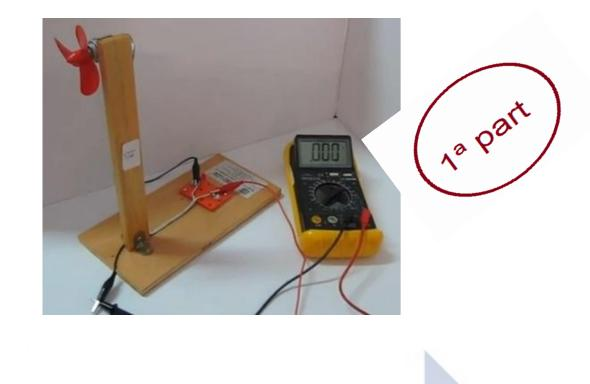
wind energy input Conversion of wind energy to mechanical energy Conversion of mechanical energy to electrical energy
